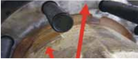
STEP 1 Clean bare hub pilots, inspect for wear, and lubricate pads.
