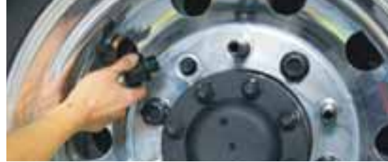
STEP 7 Install the nuts by hand.
