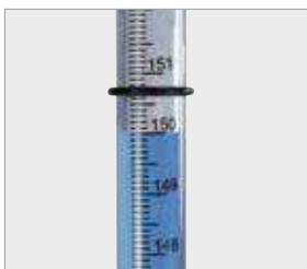
Testing scale up to 150 mbar on transparent extending tube element
